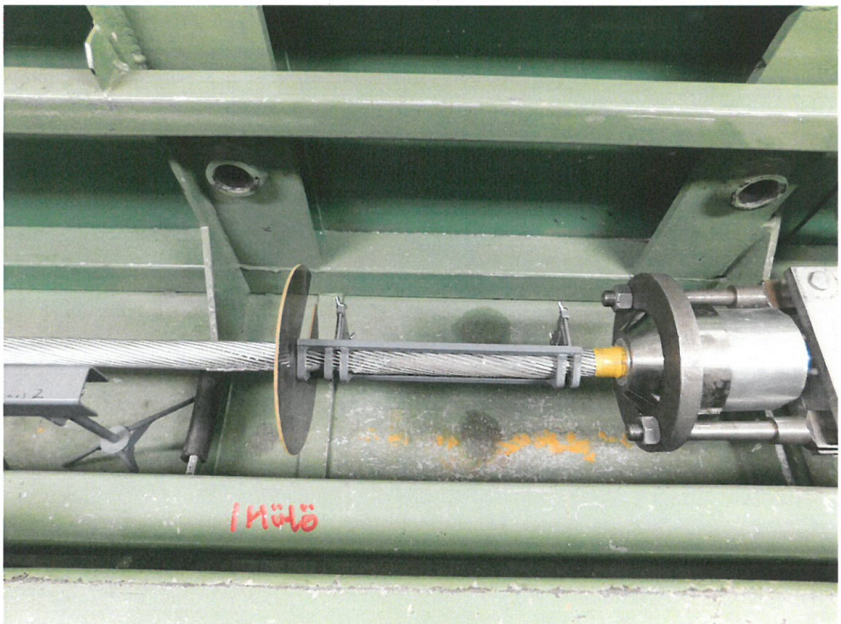
Photo 2 Conical epoxy resin end fitting used for the mechanical tests
